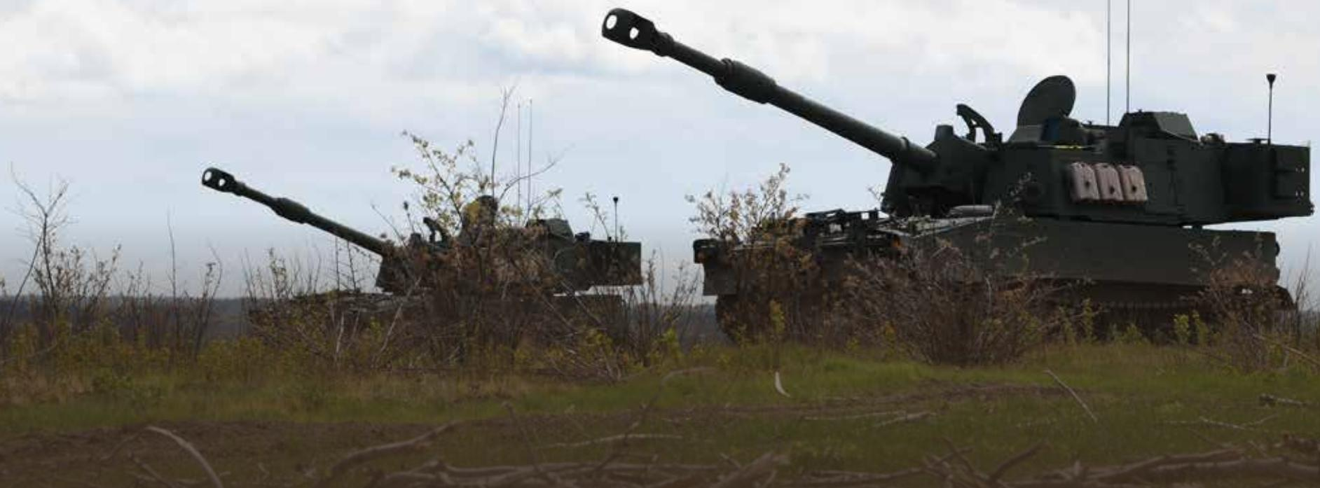
sent into battle along with ammunition or support vehicles. Today, the M109A7 uses the existing main armament and cab structure of the M109A6. It replaces the vehicle's chassis components, including the engine, transmission, final drives, suspension, and track with modern components common to the M2/M3 Bradley Infantry Fighting Vehicle. The commonality with other unit systems reduces sustainability costs while improving chassis structure and survivability.
